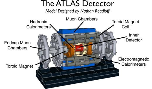
ATLAS is a general-purpose particle detector at the Large Hadron Collider (LHC) at CERN, with a broad physics programme ranging from studying the Higgs boson to searching for supersymmetry and extra dimensions. Measuring 46m long and 25m tall, it is the largest of the four detectors and sits in a cavern almost 100m underground.
